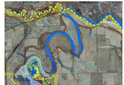
Illustration of a floodplain based on topography and estimated flood elevation.
